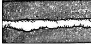
Poor Weld Appearance Arc Weld Troubleshooting
