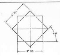
REPRODUCE THE OVERLAPPING SQUARES FULL-SIZE ON THE CENTER LINES PROVIDED BELOW. USE VISIBLE LINES, HIDDEN LINES AND CENTER LINES TO COMPLETE THE FIGURE. DO NOT DIMENSION THE DRAWING.
