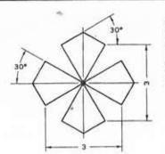
REPRODUCE THE EMBLEM DESIGN FULL-SIZE ON THE CENTER LINES PROVIDED BELOW. ALL THE INCLINED LINES ARE EITHER 30° FROM THE HORIZONTAL OR 30° FROM THE VERTICAL. USE VISIBLE AND CENTER LINES TO COMPLETE THE FIGURE, DO NOT DIMENSION THE DRAWING.
